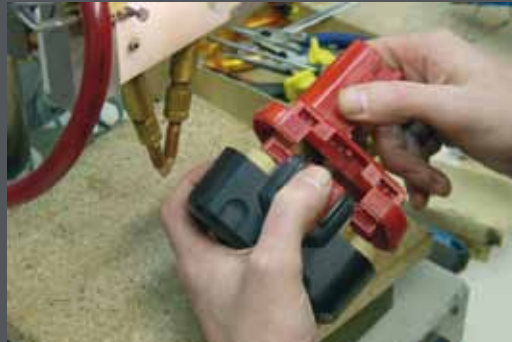
Opening the battery
